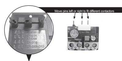
Note: The copper pins of the overload relay need to be correctly positioned to suit the contactor that it is to be mounted to.
